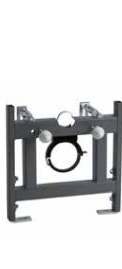
400mm Wall Hung Half Height WC/Bidet Frame 400(w) x 400(h) x 170-335(d)mm Suitable for use in narrow black to wall units including 500mm wide Use with the comfort height cistern to allow wall hung parts to be set at higher position 200mm height adjustment
